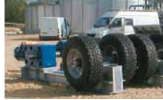
Chassis built as standardised units with Direct Drive. Without V-belt transmission.
