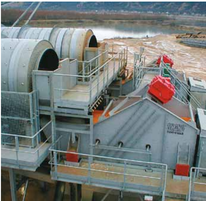
Dewatering Screens combined with after washing for very sticky materials.
