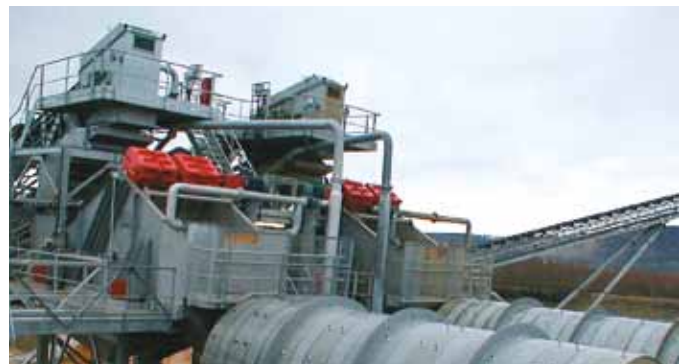
Additional screens, for removal of sand before the washing drum, or afterwards for final washing, rinsing and water removal.
